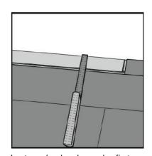
Last row (and perhaps also first row) min. width 50mm. Remember the abt 10 mm distance to wall! Cut the panels lengthwise and glue the short ends.
