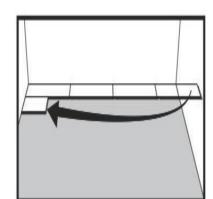
Second row. First plank minimum 300mm. Put a distance to the wall abt 10mm thick.
