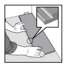
Start in the left-hand corner of the room. Place a distance about 10mm thick to the left and position the plank to the wall (tongue face into the room).
