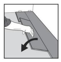
Fold down in a single action with a slight press to the short end of the previous. During fold down make sure the panels are tight against each other.
