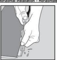
Cut of the vertical locking part of the stripe with a chisel.
