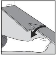
At the end of 1st row put a distance abt 10mm to the wall and measure the length of the last plank to fit.
