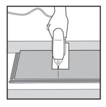
Cut with a jig saw hardwood face turned down or with a handsaw with hardwood face up.
