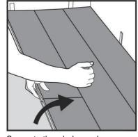
Seperate the whole row by carefully above the joint. Fold up and release the whole long side.
