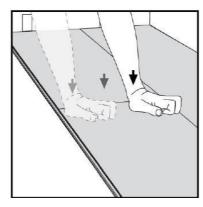
Press or knock slightly along the short end of the installed panel.
