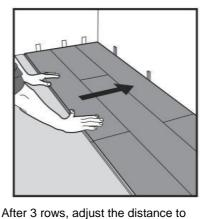
the front wall by placing distances abt 10mm to wall.
