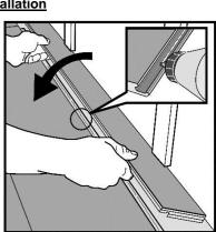
Put an applicable glue on the stripe an push the planks horizontally together. If necessary place some spacers between last board and the wall during the hardening.
