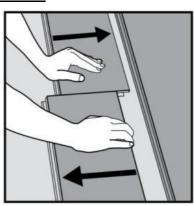
Disassemble the panels by sliding the short ends horizontally. Do never fold up a panel, as this will damage the profile.
