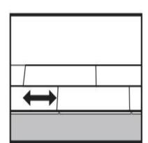
General: Minimum distance between short ends of planks in parallel rows shall not be less than 300mm.
