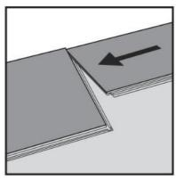
Place 2<sup>nd</sup> plank gently and tight to the short end of 1<sup>st</sup> plank. Fold down the panel in a single action movement. During the fold down make sure the panels are tight against each other. Afterwards press or slightly knock at the short end just installed.
